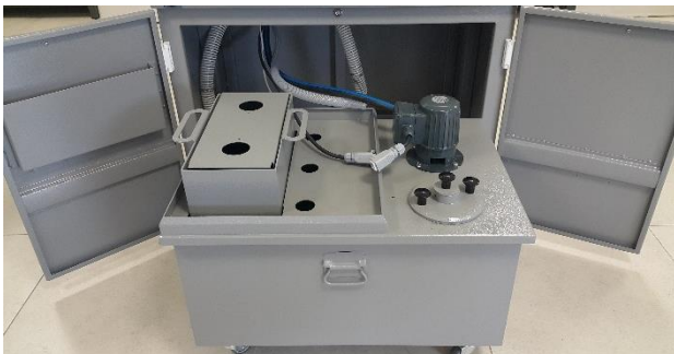
Recirculation Cooling Tank
