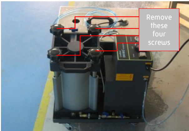
Opening the Filtering Tank
