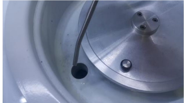
Cleaning of the Drain Hole
