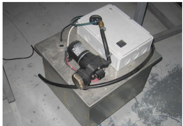
Recirculating Cooling System
