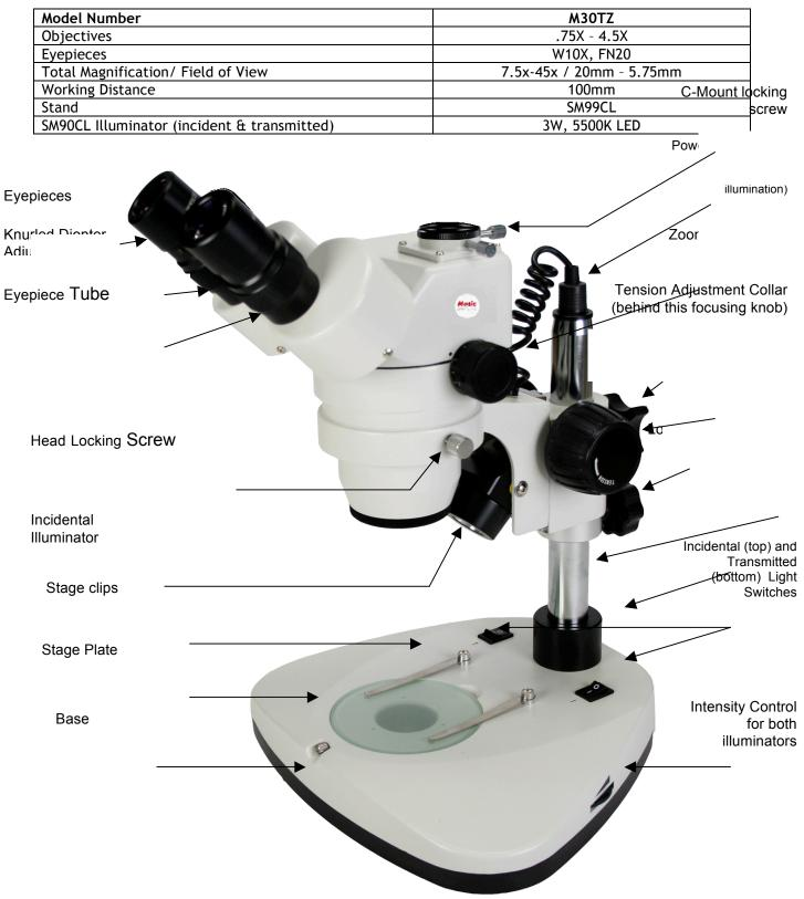
Stereoscopic microscopes are designed for viewing 3-dimensional objects, inspection, or assembly of small parts, and for dissection of biological specimen at low magnification. The 45° inclined viewing head provides an upright, unreversed image which permits easy manipulation of object being viewed while looking through the microscope. The incidental and transmitted illuminators incorporate high intensity 3 watt LED lamps.
