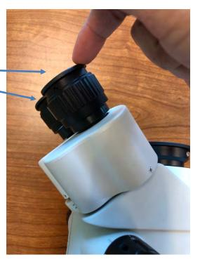
II. Pull the dust cap off that is covering your trinocular port.
