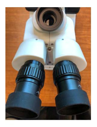
5. Next, using a 3mm size allen wrench, loosen the two silver screws on either side of the top of the trinocular port of the microscope.
