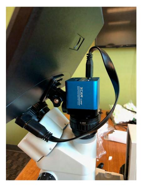
17. Next, take the end of your camera power supply and insert it into the single end of the splitting adapter.
