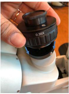
7. Once resting, re-tighten both silver set screws on the trinocular port so that the adapter is secured tightly in place.
