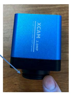
10. You'll then screw the camera onto the threads of the C-Mount adapter until the camera is stable (be careful not to overtighten the camera).
