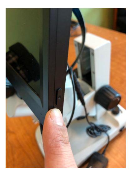
22. The on/off button for the illuminators of the stand is on the right hand side of the base of the stand.
