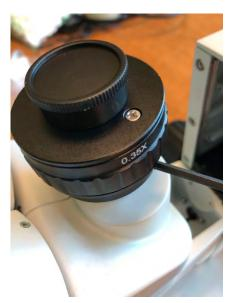
8. There is a dust cap on the C-Mount adapter that you'll want to remove by unscrewing it.
