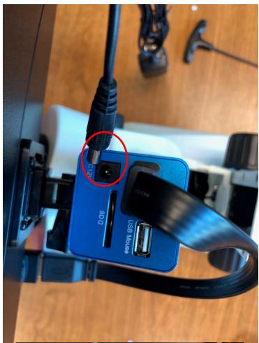
Take the other end and insert it into the "DC-12V" port on the monitor
