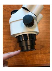
3. Next, insert the body of the microscope into the focusing holder of the stand. Once resting in the focusing holder, you can re-tighten the silver set screw on the focusing holder.
