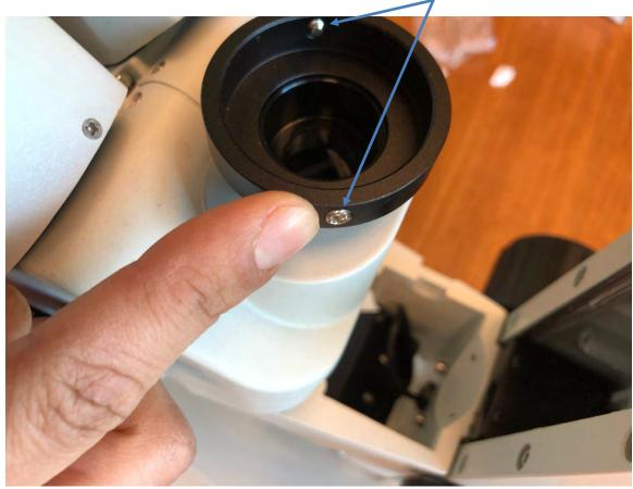
6. Next, insert the C-Mount adapter into the trinocular port so that it is resting level.
