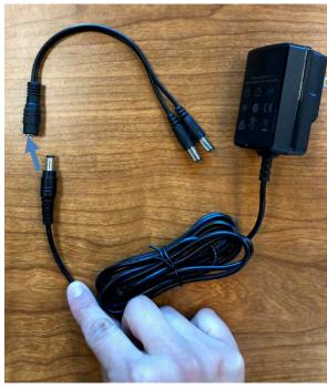
18. Take one end of the splitter and insert it into the "DC12V" port on the camera.
