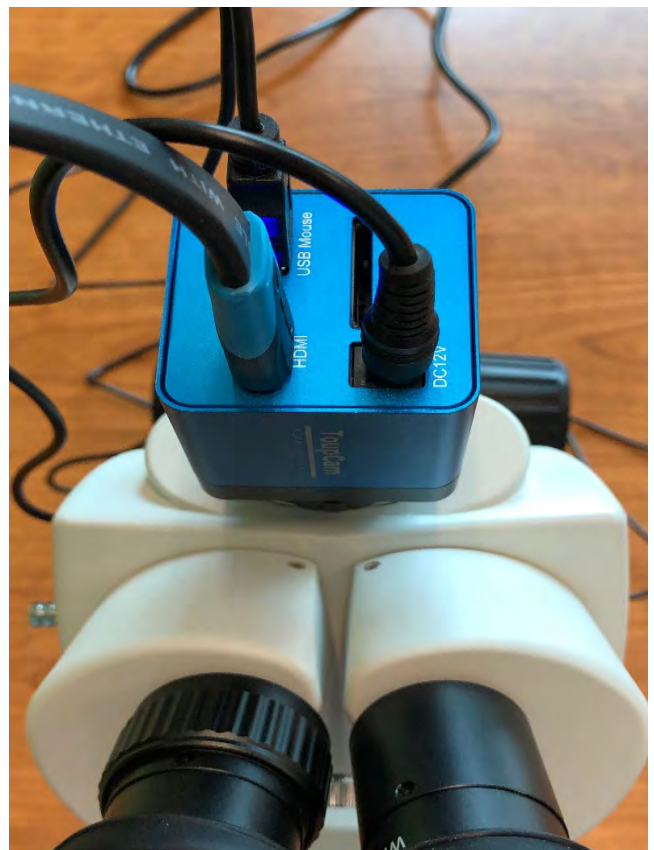
Image of all cables connected to the camera
