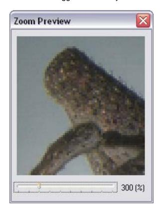
The zoom preview window is a floating window created automatically by INFINITY ANALYZE upon startup. It magnifies a small region of an image. The magnification rate is adjustable with the slider at the bottom of the zoom preview window. The zoom preview window works on both still image and live image. The region to magnify is set by current mouse position.
