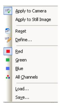
The LUT menu is accessed from the File -> Lookup Table menu. Each function represented with an icon beside has been explained in the table above. Use the Apply to Still Image option on this menu to apply the LUT to the active image in the ANALYZE working area. Use the Load... and Save.. options to restore or save an LUT definition.
