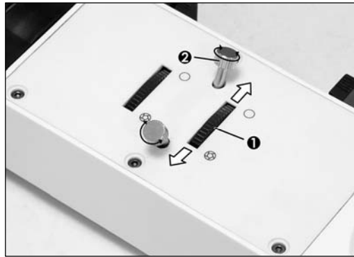
1. Field Diaphragm Adjustment Wheel 2. Field Diaphragm Centering Screw
