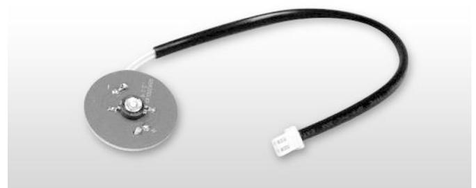
6. Feed LED cable through LED board locating ring.
