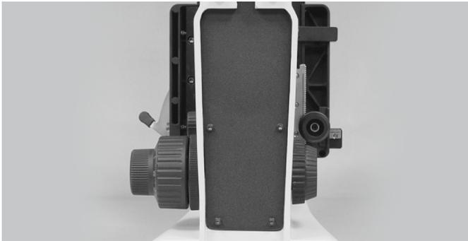
2. Unscrew four Allen hex socket cap screws holding back cover plate.
