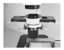
• Stopping down the aperture diaphragm will lower the resolution and brightness but increase the contrast and depth of focus. By stopping down the N.A. of the condenser to 2/3 of the N.A. of the objective, a good image of suitable contrast will be obtained.
