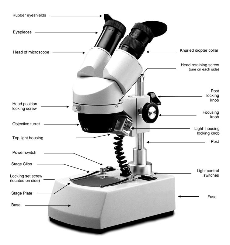
Stereoscopic microscopes are used for viewing 3-dimensional objects, inspection or assembly of small parts, and for dissection of biological specimen. They provide an upright, unreversed image which permits easy manipulation of the object being viewed while looking through the microscope. They are designed for viewing solid objects at low magnification, but they will also permit viewing of some transparent specimen slides.
