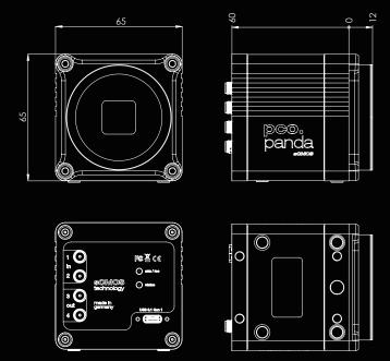
F-mount and C-mount lens adapter are changeable. All dimensions are given in millimeter.
