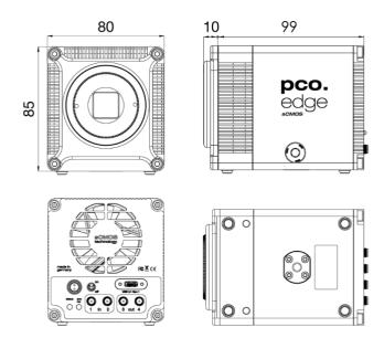
All dimensions are given in mm. Lens mount adapters are changeable. Detailed drawings are available at www.pco.de on request.
