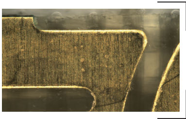
Ring Light illumination with glare removal (details on the edges now visible)
