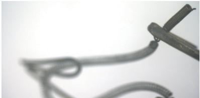
Light Bulb Filament inspected by classic microscope
