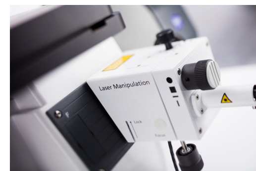
Use Laser Manipulation with DirectFRAP to analyze fast intracellular processes.
