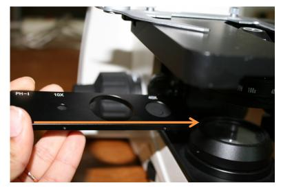
• Not all phase contrast microscopes are the same but generally they rely on similar techniques to set up the system for optimum results. In the system shown below, the condenser has 5 settings, 4x, 10x 40x, 100x, PH. 4x-100x are for your brightfield settings with no Phase. Move your slider to the PH setting when using the 40x Phase lens.
