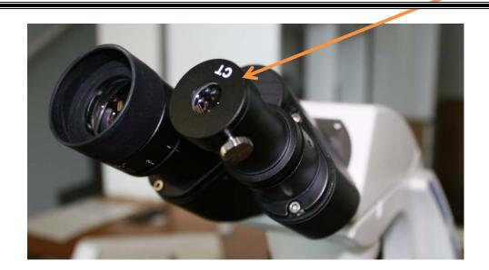
• When looking through the centering telescope, you will see two rings. They may or may not be concentric. By using a small allen wrench, you center the 40x ring on the phase slider so that the rings you see when looking through the telescope are concentric (see the image below).
