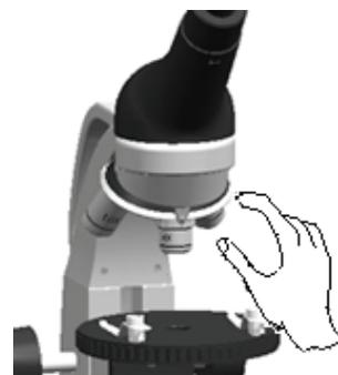
Focus by first adjusting the coarse focus knob, and then the fine focus knob.
