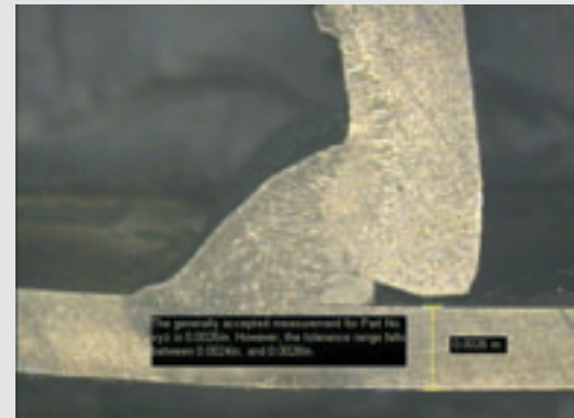
Overlay allows you to compare live image Leg #1 thickness with the standard for quick visual analysis.
