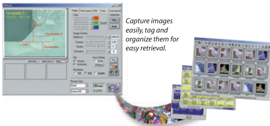
Overlay allows you to compare live image Leg #1 thickness with the standard for quick visual analysis.
