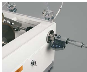
Precise micrometer with digital readout
