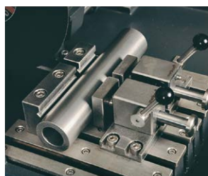
Stainless steel clamping devices and T-Slotted table
