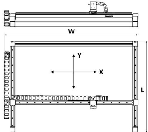
Comprised of custom cut linear guiding system mounted on high density aluminium profile for smooth and stable XY-travel of digital camera. The system is fitted with mounting brackets to allow the correct setting of working distance during installation in the user's rack system. Removeable front profile for extension of the field of view. 4-direction tilt unit, Z-extender bracket and camera grip handle are available for XY-travel Stand as extra accessories.
