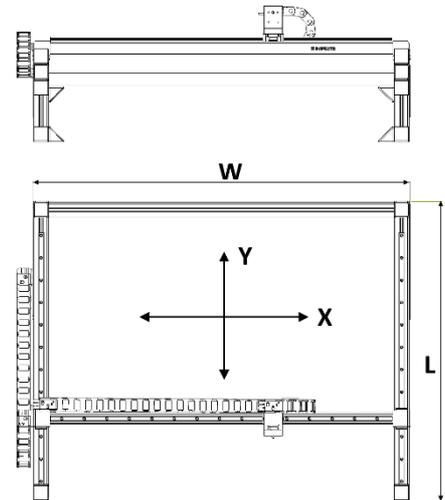
Comprised of custom cut linear guiding system mounted on high density aluminium profile for smooth and stable XY-travel of digital camera. The height of the linear guide can be adjusted and set for desired working distance of the Digital Microscope. 4-direction tilt unit, Camera grip handle, and Z-extender brackets are available for XY-travel Stand as extra accessories.
