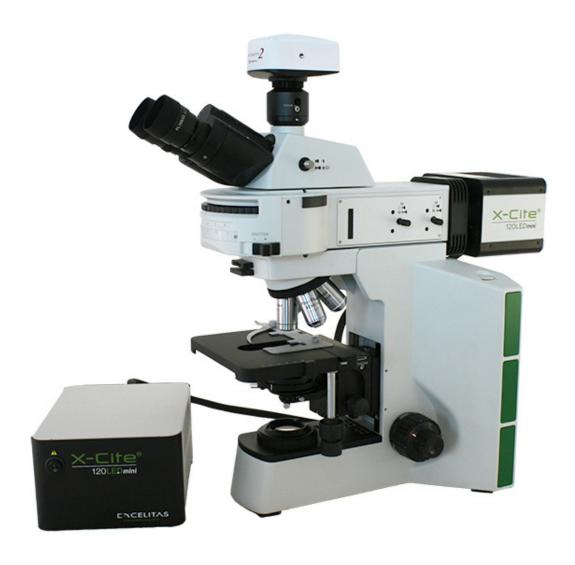
Fluorescence illumination attachment with six position filter turret. Illuminator options include metal halide illuminator with liquid light guide and collimating adapters or LED illuminator.
