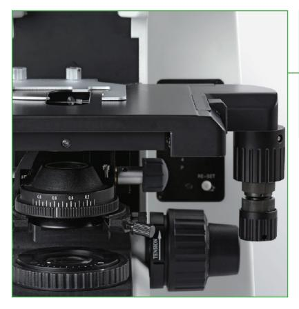
Double-layer mechanical stage, 187 x 168mm. Dual slide holder can hold one or two slides for testing and comparative analysis. Right hand ergonomic controls for X-Y axis travel of 80 x 55mm with precision of 0.1mm. Stage is made of oxidized metal with a special anti-corrosive protective coating providing durability and ease of cleaning.
