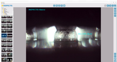
BGA bump (high magnification)
