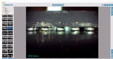
BGA bumps (large field of view)
