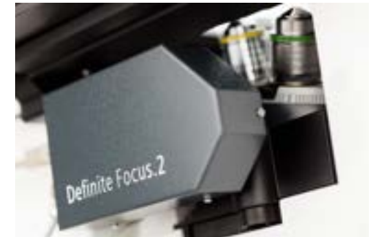
Definite Focus.2 is integrated into the nosepiece of your Axio Observer 7.
