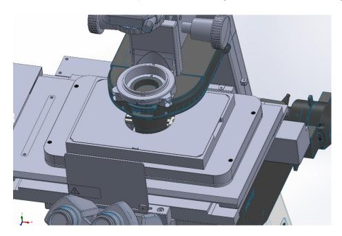
Installation of the Nikon TI laser safety adapter kit QGSPADAPT1-TI-LSC is now complete.
