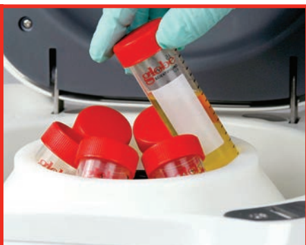
Twelve position rotor compatible with 15mL and 50mL conical tubes
