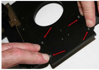
8. On the focusing holder locate the four holes that will match up with the mechanical stage shown above.
