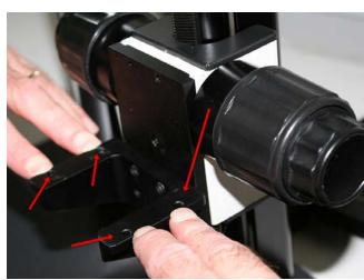
9. Screw the four screws into the mechanical stage from beneath the stage using the allen wrench.
