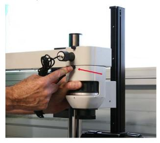
11. Connect the stereo microscope head and tighten the set screw.
