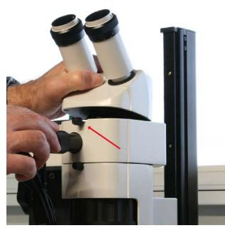
12. Connect the observer head and tighten the set screw.
