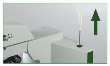
Allen wrench storage in microscope frame ensures you can always locate the required tool for microscope adjustments.
