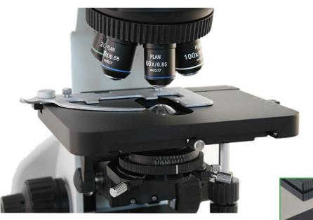
Double-layer mechanical stage, 175 x 145mm. Dual slide holder can hold one or two slides for testing and comparative analysis. Right hand ergonomic controls for X-Y axis travel of 75 x 50mm. Stage is made of oxidized metal with a special anti-corrosive protective coating providing durability and ease of cleaning.
