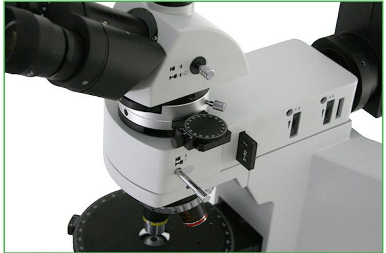
Intermediate device for professional conoscopic observation has internal Bertrand lens, analyzer, and slot for full  $\lambda$  plate,  $1/4 \lambda$  plate and quartz wedge.
